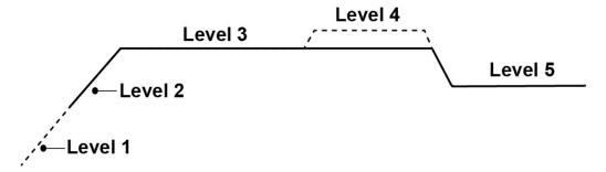
**Soft Charge-** When batteries suffer an over-discharge, the controller will softly ramp the battery voltage up to 10V.
