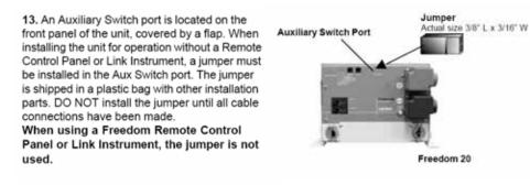
Current versions of the product do not require the installation of the jumper, because it is no longer necessary for operation of the inverter when used without a remote control. The Auxiliary Switch Port can now be used to turn the inverter on with the use of a contact closure. Connecting these two pins together turns the inverter on, and disconnecting them turns the inverter off. Some RV manufacturers use this feature to power a back-up camera and a 120 Volt TV.
