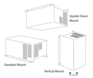
This versatile deck mount converter can be installed in any position, making RV design more ° exible for manufacturers. Mount converter vertically with fan at the bottom to enhance cooling. WF-8800 Series converter features easy horizontal installation and can even be installed upside down.
