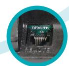
The EM-20 allows a simple remote control hook up for convenient end-user power management.
