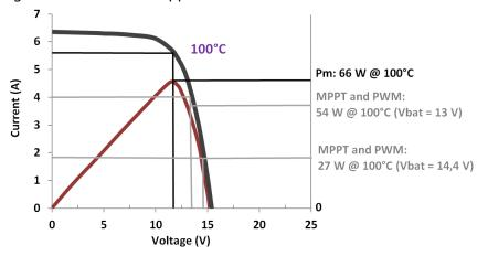
Fig 12: At 100°C panel temperature the Maximum Power Point voltage is 11.7 V
