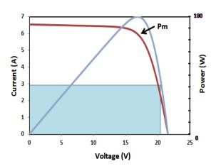
Fig 4: Less power harvested: voltage is too low
