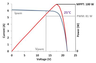
Fig 7: PWM charge controller
