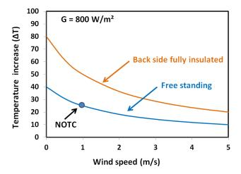
Fig 17: Wind speed and temperature increase
