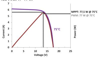
Fig 11: Comparison of MPPT and PWM performance at 75°C panel temperature Black lines: MPPT (77.5 W).
