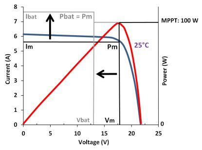
Fig 6: MPPT controller, graphical representation of the DC to DC transformation  $Pm = Vm \times Im = 18 \text{ V} \times 5.6 \text{ A} = 100 \text{ W}$ , and  $Pbat = Vbat \times Ibat = 13 \text{ V} \times 7.7 \text{ A} = 100 \text{ W}$
