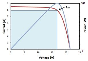
Fig 2: Current-voltage curve (brown) and power-voltage curve (blue,  $P = V \times I$ )
