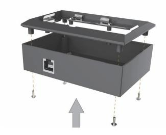
**Step 3:** assemble the wall mounting box to the wall
