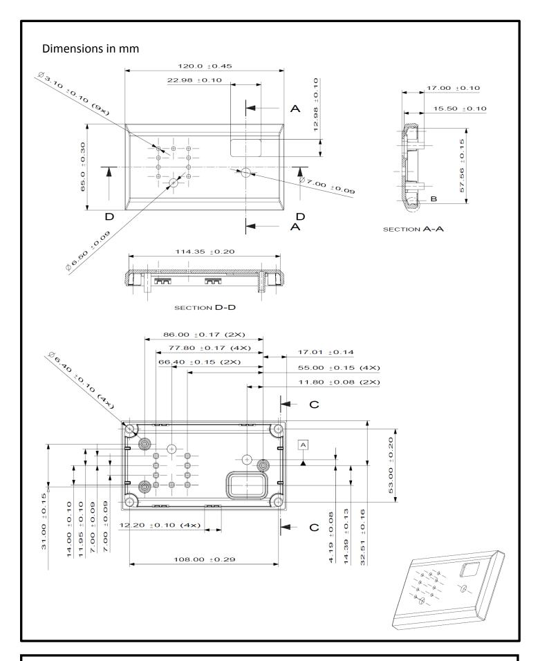
Dimensions of plastic panel DMC000200000R Digital Multi Control 200/200A GX
