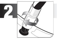
Attach the end of the air hose to the valve stem on your tire
