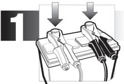
Attach the alligator clamps to the battery. Remember: Red to Positive and Black to Negative. Make sure the compressor is in the off (O) position prior to attaching the battery clamps.
