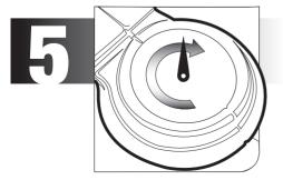
To check tire pressure, manually turn the compressor off. Once the gauge settles, that will be the accurate pressure in the tire.
