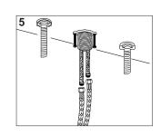
**5.** CONNECT WATER SUPPLY Connect existing water supply lines to the faucet supply lines.
