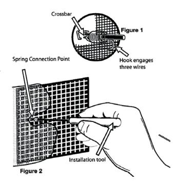
Cleaning the screens is necessary for proper air flow. Inspect screens frequently and clean as needed. Save the installation tool for reinstallation of screens after cleaning.
