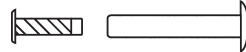
20-183 Rivet and Drive Screw Assy. Used when no rivet tool is available.
