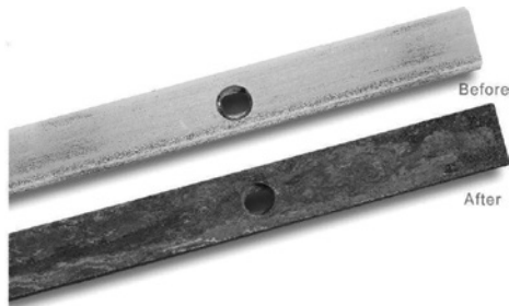
3,000 hours Salt Spray Test Stainless Steel
