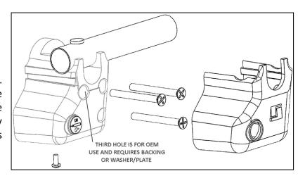
provided to add stabilization for the rail. If no stud is available at mounting hole locations, you may have to drill through the wall of the coach and use large washers/backer plates for load distribution.
