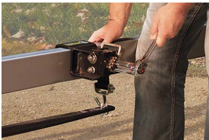
Straptek adjusts by simply tightening or loosening the heavy-duty polyester straps with a standard socket wrench, saving time and energy.
