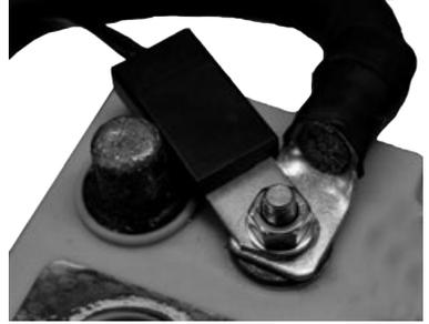
Fig 2.5(b) Temperature Sensor Installation
