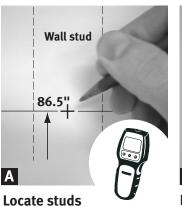
On closet wall, locate all wall studs and mark them 86.5" above the floor. Using a stud finder can be useful (optional).
