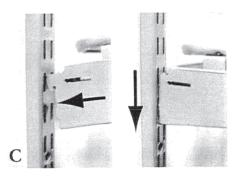
Angle Brackets into Upright slots and push down on both Brackets to lock into place. Securely tighten screws from Step B. Note: If Brackets do not line up with slots in the Uprights, loosen screw(s) on Uprights before installing. Once installed, retighten screw(s) in Uprights.
