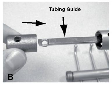
Insert Bar Lock onto Tubing Guide.
