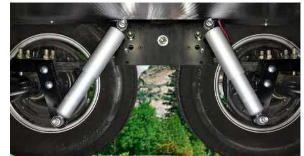
The complete Comfort Ride system (above) includes shock absorbers and slipper leaf springs.
