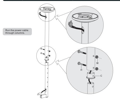
Insert plastic bushing and inner column into the outer column and fix them at the desired height using the correct combination of screw and nut.
