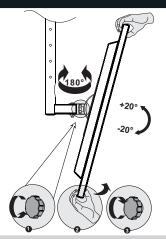
Use the tilt adjusting knob to adjust your display to the desired angle then tighten it.
