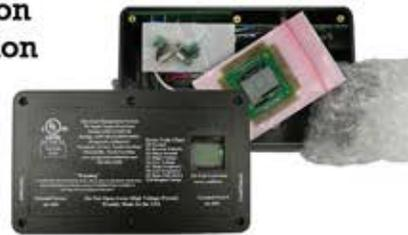
The EMS-LCHW units are shipped with the digital display and extra hardware tucked **INSIDE** the unit for safe shipping. Simply remove the lid.
