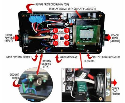
NOTE: Only one (1) wire through each sensor. Black wire goes through curent sensor (with green tape) to T1.
