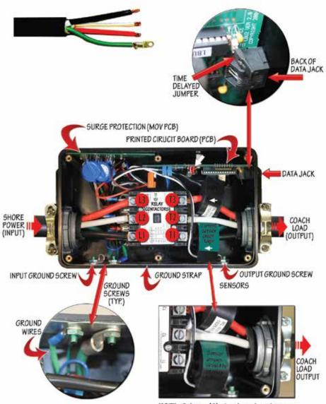
**NOTE:** Only one (1) wire through each sensor. Black wire goes through curent sensor (with green tape) to T1.
