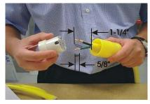
**4.** Strip outer jacket of cord 1-1/4 in. and 5/8 in. of insulation off each of the three wires. Cut away filler. Make sure the wire is clean and with bright copper color. Do not solder the ends of the wire.
