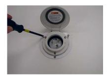
Position the gasket and inlet over the adapter mounting bracket. There are two brackets provided. Choose the appropriate mounting bracket based on the size of the hole. Align the mounting holes and tighten the screws to 5-7 in.lbs. torque with provided 8-32 screws. Fasten the mounting bracket to existing mounting holes.
