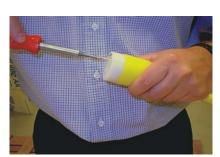
7. Tighten down the recessed screws with moderate torque.
