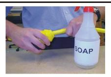
2. Push cord through the inverted end about 12 in. A tug in the opposite direction returns boot to its original shape.
