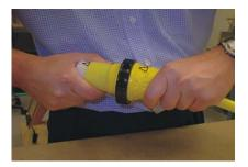
**9.** Align device and boot indicators and lubricate mouth of boot and rear shoulder of device with soap solution and pull into place. Be sure boot is on as far as it will go.
