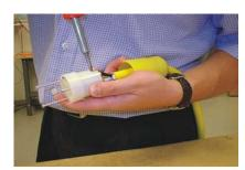
**5.** Insert bare wires into their corresponding color-coded terminals. Make certain there is no wire insulation under any terminal clamp. Tighten the screw clamps to 14-20 in.-lbs torque.
