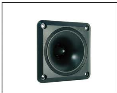
NTX-3535PZ 3.5" X 3.5" TWEETER • Frequency Range: 2.3K~20KHz • Power RMS/Max: 75/150W • Impedance: 4-8 Ohms • Mounting Diameter: 73mm
