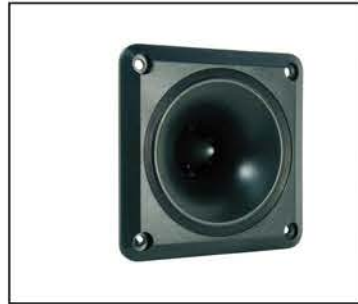
NTX-1033PZ PIEZO TWEETER 3" SQUARE • Frequency Range: 5K~20KHz • Power RMS/Max: 75/150W • Impedance: 4-8 Ohms • Mounting Diameter: 58mm
