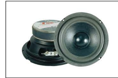
NWX-623-8 6.5" PAPER CONE • Frequency Response: 70Hz-13000Hz • Power RMS/Max: 65/130W • Impedance: 8 Ohms • Mounting Diameter: 156*4-5.8
