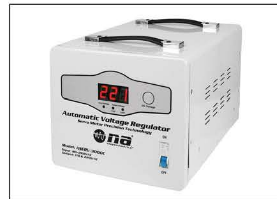
ASERV-3000C 3KVA AUTOMATIC VOLTAGE REGULATOR • Servo Motor Transformer • Wide Input Voltage Range: 80-260V • Dual Output: 110V AC and 220V AC at the Same Time • Advanced CPU Control Circuit • Automatic 10 Second Countdown Delay Function Integrate • Full Protection Design: High Voltage/Low Voltage/High Temperature/Short Circuit • Accurate Output Regulation: \pm 3\%
