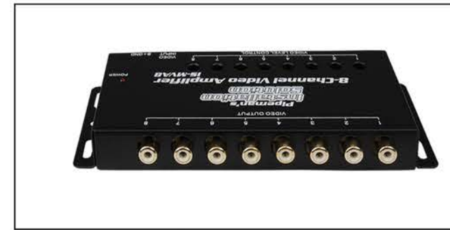
IS-MVA8 8-CHANNEL VIDEO AMPLIFIER • Each Channel Output can be Independently Adjusted • Shielded Metal Housing • Power Supply Voltage: 12V • Output Impedance: 75Ω • Video Level: Input: 1.0Vp-p / Output: 0.5-1.5Vp-p
