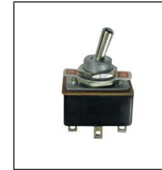
EC-1501 TOGGLE SWITCH CENTER-OFF • D.P.D.T. Center-Off Toggle Switch • Mount Size : 12/25" • 117V AC • 3 Amp • 6 P
