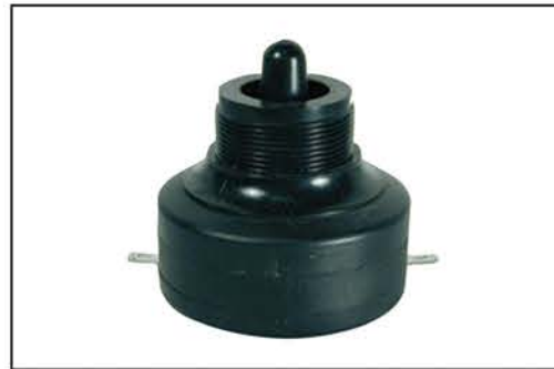
NTD-100 PIEZO DRIVER SMALL • Frequency Response: 3.5-20KHz • Impedance: 4-8 Ohms • Power RMS/Max: 37.5/75W
