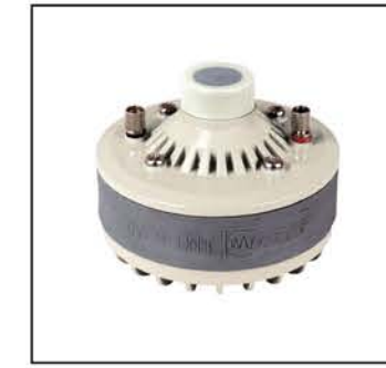
NAD-100 100 WATTS DRIVER UNIT IVORY • Frequency Response: 180-500Hz • RMS/Max Power: 100/200W • Impedance: 16 Ohms • Voice Coil: 51.6mm (2") Til
