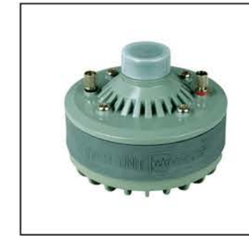
TD-100 DRIVER UNIT • Rated Input: 100W RMS / 200W Max • Impedance: 16 Ohm • S.P.L. (1W/M): 110 dB • Frequency Response: 180-5000 Hz • Voice Coil: 51.6mm (2") til • Magnet: 120 x 60 x 20 mm
