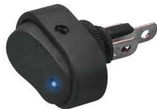
IS-EC-OVL12-BLU 12V DC 20AMP OVAL BLUE LED LIGHT ILLUMINATED 3P ROCKER SPST ROCKER TOGGLE SWITCH • Easily Fits in 12mm Diameter Opening • Designed to Connect and Disconnect an Electrical Circuit at will - Applicable for Car, Motorcycle, Boat, UTV, RV Etc. • Lower LED is Independent and can be Wired to Separate Dash Light Circuit • Material: ABS • LED Light Color: Blue
