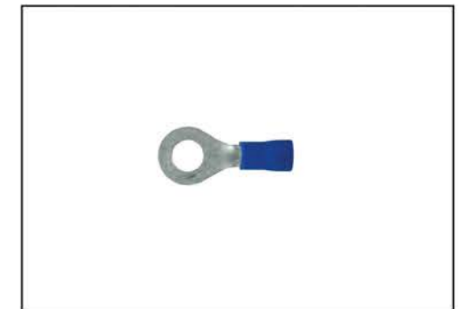
IS-RT-1614-516 VINYL RING TONGUE TERMINAL • Pack of 100 • 16-14 Gauge • Stud Size #5/16 • Insulated • Blue
