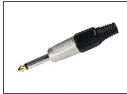
X-1132BK • 1/4" • Mono Male • Nickel Finish • Gold Tip • Connects Cable which is between Ø 6~7mm • Black Color
