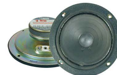
NMX-516-8 5" MIDRANGE 100 WATTS • Frequency Response: 500-10KHz • Power RMS/Max: 15/30W • Impedance: 8 Ohms • Mounting Diameter: C 124.5-4- C 4.5
