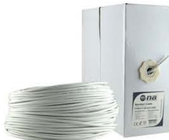
CABLE 16CL2-500 IN-WALL SPEAKER CABLE • 2 x 16 AWG • Copper Clad Aluminum Conductors • White PVC • CL2 Rated for In-Wall Installation • Length: 500'
