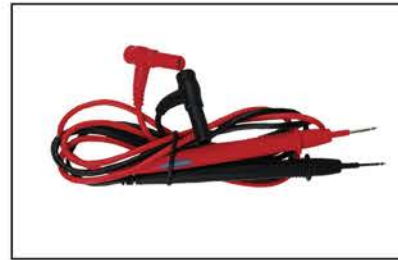
NB-437 TEST LEADS SET • Flexible cable with right angle DMM plugs • 0.08" (2mm) diameter contact tips • Max Test Voltage: 600V/1000V • Max Test Current: 10A
