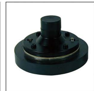
NDX-6740 40 OZ. DRIVER • Voice Coil: 1-1/2" (38mm) Aluminum • Impedance: 8 Ohms • Magnet: 40 Oz. • Power RMS/Max: 200/400W • Mounting Diameter: 34mm
