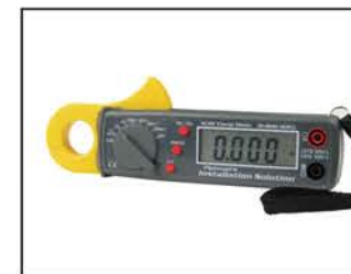
IS-HHM-16DCI • DCV: 0-1000V \pm (1%+1) • ACV: 0-750V \pm (2%+3) • DCA: 0-200A \pm (2%+3) • ACA: 0-200A \pm (2.5%+3) • OHM: 0-40m \Omega \pm (1.5%+2) • Continuity Beep • Frequency Test • Capacitance Test • Diode Test
