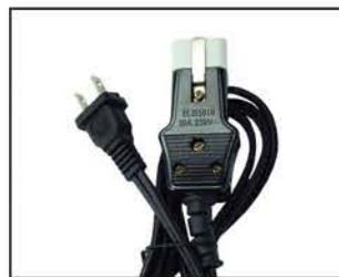
CMC-200 APPLIANCE ELECTRICAL CORD • Connector made of ABS and Bakelite for Resistance to Extreme Heat • Cable: 2*38*0.14 CCA • OD:3.8*7.6 • 10A 250V • 6FT
