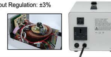
ASERV-1000C 1KVA AUTOMATIC VOLTAGE REGULATOR • Servo Motor Transformer • Wide Input Voltage Range: 80-260V • Dual Output: 110V AC and 220V AC at the Same Time • Advanced CPU Control Circuit • Automatic 10 Second Countdown Delay Function Integrate • Full Protection Design: High Voltage/Low Voltage/High Temperature/Short Circuit • Accurate Output Regulation: \pm 3\%
