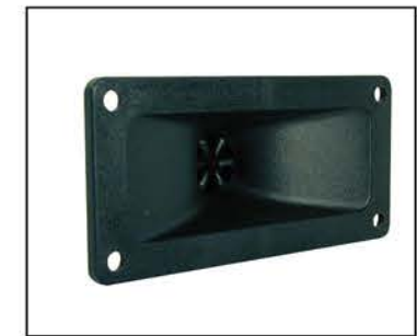
NTX-1015PZ 2X5 PIEZO 75W TWEETER • Frequency Range: 3K~40KHz • Power RMS/Max: 37.5/75W • Impedance: 4-8 Ohms • Mounting Diameter: 121mm x 43mm
