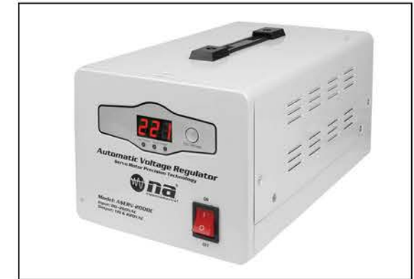
ASERV-2000C 2KVA AUTOMATIC VOLTAGE REGULATOR • Servo Motor Transformer • Wide Input Voltage Range: 80-260V • Dual Output: 110V AC and 220V AC at the Same Time • Advanced CPU Control Circuit • Automatic 10 Second Countdown Delay Function Integrate • Full Protection Design: High Voltage/Low Voltage/High Temperature/Short Circuit • Accurate Output Regulation: \pm 3\%
