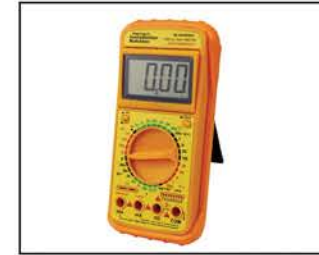
IS-HHM95 • DCV: 0-2-20-200-1000V (1M \Omega ) \pm 0.5% • ACV: 0-200m-2-20-200-750V (450K \Omega ) \pm 1.2% • DCA: 2m-20m-200m-20A \pm (0.8% + 3) • ACA: 2m-20m-200m-20A \pm (0.8% + 10) • Impedance: 10m \Omega • Continuity Beep • Indicated Over Range • Diode Test
