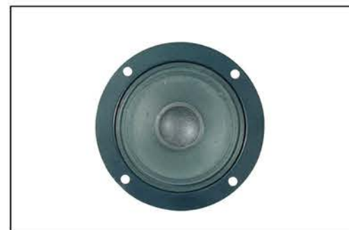
NTX-3R 3.5" ROUND SPEAKER • Frequency Response: 2K-18K Hz • Power RMS/Max: 10/20W • Impedance: 8 Ohms • Mounting Diameter: \varnothing 89-4- \varnothing 5
