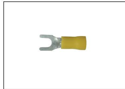
IS-SP-1210-10 VINYL SPADE TERMINAL • Pack of 100 • Insulated • 12-10 Gauge • # 10 Stud Size • Yellow
