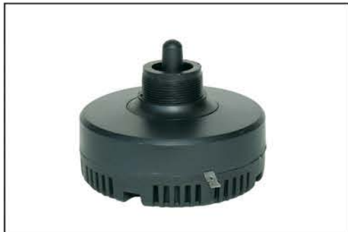
NTD-350 PIEZO DRIVER LARGE • Frequency Response: 1.5-22KHz • Impedance: 4-8 Ohms • Power RMS/Max: 50/100W
