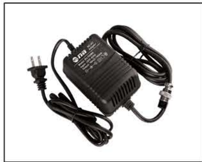
DV-700MX AC POWER ADAPTER • Current: 700mA • Input: 120V, 60Hz • Output: 18V
