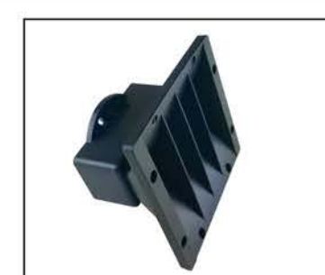
NTX-6464-WV 6.33" x 6.33" PLASTIC HORN • Frequency Range: 3K~30KHz • Power RMS/Max: 60/120W • Impedance: 4-8 Ohms • Mounting Diameter: 146mm x 85mm
