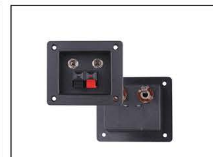
TCR-200 SPEAKER TERMINAL • Size: 3-1/4" x 4" • Type: 2 1/4" Jacks without Crossover
