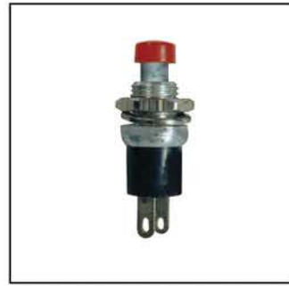
NB-602PD MOMENTARY PUSH BUTTON • Push to Deactivate • Current Rating: 3A 125V AC • 2 Pins
