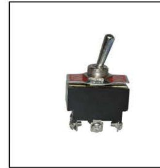
EC-1500 TOGGLE SWITCH CENTER-OFF • D.P.D.T. Center-Off Toggle Switch • Mount Size : 12/25" • 117V AC • 6 Amp • 6 P
