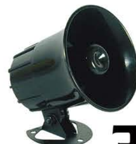
AV-1006 SIREN OUTPUT: 119 DB • 4" 6 Tone Siren • Operation Power: 12V, 35W • Sensitivity: 119dB± 3db • Impedance: 8 Ohms
