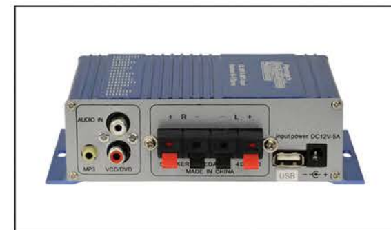
IS-AMP-220 HIFI STEREO AUDIO AMPLIFIER • Input: DC 12V, 5A • Power: 20W Max, 10W RMS • Speaker Impedance: 4~16Ω • Frequency: 20Hz~20KHz
