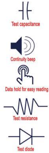
IS-HHM95 • DCV: 0-2-20-200-1000V (1M \Omega ) \pm 0.5% • ACV: 0-200m-2-20-200-750V (450K \Omega ) \pm 1.2% • DCA: 2m-20m-200m-20A \pm (0.8% + 3) • ACA: 2m-20m-200m-20A \pm (0.8% + 10) • Impedance: 10m \Omega • Continuity Beep • Indicated Over Range • Diode Test
