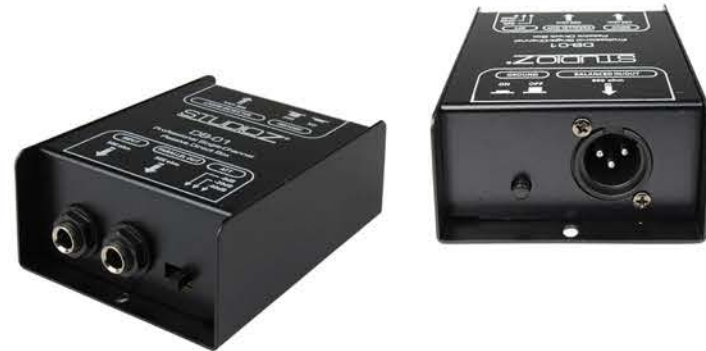
DB-01 PROFESSIONAL SINGLE-CHANNEL PASSIVE DIRECT BOX • Input Attenuation: Switchable (0dB, -20dB, -40dB) • Instrument Input: 50K Unbalanced TS Jack • Parallel (Link) Out: 50K Unbalanced TS Jack • Balanced Output: 600Ω Balanced XLR Jack • Ground Lift: Switchable Ground Lift • Construction: All Steel Chassis • Dimensions: 4.7" x 3" x 1.8" (120 x 76.5 x 45mm)
