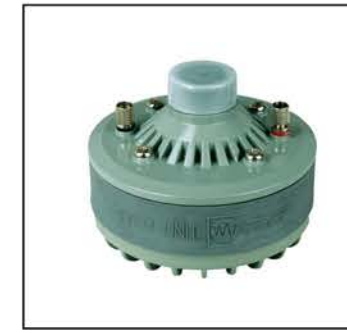
TD-60 DRIVER UNIT • Frequency Response: 180-5000Hz • RMS/Max Power: 60/120W • Impedance: 16 Ohms • Voice Coil: 51.6mm (2") Til
