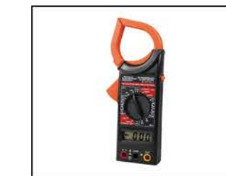
IS-HHM26ACI Digital Multimeter with AC Clamp Meter • DCV: 0-1000V \pm (0.5% + 1) • ACV: 0-750V \pm (1% + 4) • ACA: 0-1000A \pm (2% + 5) • OHM: 200-20K \Omega \pm (2% + 2) • Continuity Beep • Maximum Display: 1999 • Does Not Include Battery
