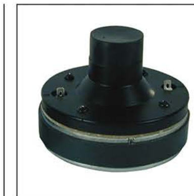
NDX-6720 20 OZ. DRIVER • Voice Coil: 1-1/2" (38mm) Aluminum • Impedance: 8 Ohms • Magnet: 20 Oz. • Power RMS/Max: 175/350W • Mounting Diameter: 34mm
