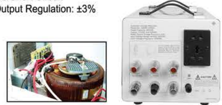
ASERV-5000C 5KVA AUTOMATIC VOLTAGE REGULATOR • Servo Motor Transformer • Wide Input Voltage Range: 80-260V • Dual Output: 110V AC and 220V AC at the Same Time • Advanced CPU Control Circuit • Automatic 10 Second Countdown Delay Function Integrate • Full Protection Design: High Voltage/Low Voltage/High Temperature/Short Circuit • Accurate Output Regulation: \pm 3\%
