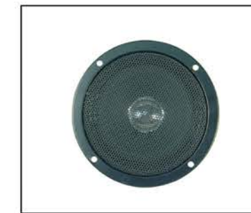
NMG-408 4" MIDRANGE 25 WATTS • Frequency Response: 1,200-15Hz • Power RMS/Max: 12.5/25W • Impedance: 8 Ohms • Mounting Diameter: C 114-4- C 5
