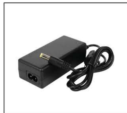
DVCA-548 AC TO DC ADAPTER • Input: AV 100~240V, 0.32~0.75A, 50/60Hz • Output: DC 12V, 5A • Power: 60W • 5 A Output • Connector Size: 5.5 x 2.5mm
