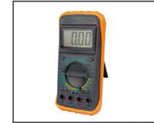
IS-HHM95TF • DCV: 0-2-20-200-1000V (1M \Omega ) \pm 0.5% • ACV: 0-200m-2-20-200-750V (450K \Omega ) \pm 1.2% • DCA: 2m-20m-200m-20A • ACA: 2m-20m-200m-20A • Impedance: 10m \Omega • Temperature Test: -40°C - 1000°C • Continuity Beep • Indicated Over Range • Does Not Include Battery
