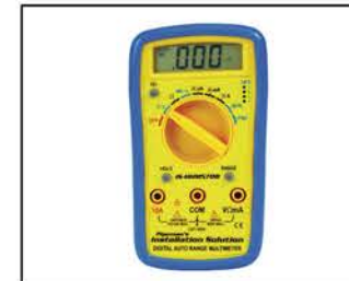
IS-HHM5708 Digital Auto Range Multimeter • DCV: 0-500V \pm (1%+2) • ACV: 0-500V \pm (1%+3) • DCA: 0-10A \pm (2%+3) • ACA: 0-10A \pm (1.2%+3) • OHM: 0-20M \Omega \pm (2%+3) • Continuity Beep • Auto Range & Power Off • Diode Test • Data Hold • Maximum Display: 1999 • Power: 3V
