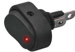
IS-EC-OVL12-RED 12V DC 20AMP OVAL RED LED LIGHT ILLUMINATED 3P ROCKER SPST ROCKER TOGGLE SWITCH • Easily Fits in 12mm Diameter Opening • Designed to Connect and Disconnect an Electrical Circuit at Will - Applicable for Car, Motorcycle, Boat, UTV, RV Etc. • Lower LED is Independent and can be Wired to Separate Dash Light Circuit • Material: ABS • LED Light Color: Red
