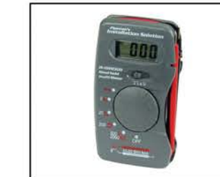
IS-HHM300 Handheld Multimeter • DCV: 2-500V \pm (0.5%+1) • ACV: 2-500V \pm (1.2%+10) • DCA: 0-200mA \pm (2%+2) • OHM: 2-2000 K \Omega \pm (1%+2) • Continuity Beep • Diode Test • Power: 12V • Dimensions: 2.8" x 4.7" x 0.7" • Weight: Approx 0.24 lb (110 g included Battery)
