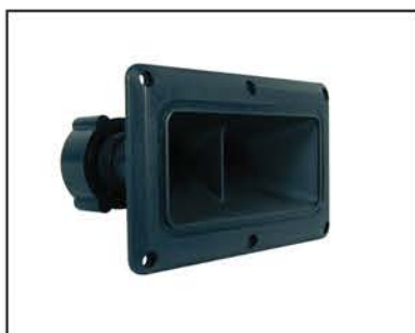
NTX-362 3" X 5" DOUBLE WIDE DISPERSION PLASTIC TWEETER • Frequency Range: 3K~25KHz • Power RMS/Max: 75/150W • Impedance: 4-8 Ohms • Mounting Diameter: 163mm x 95mm
