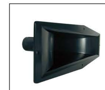
NTX-3515 PLASTIC HORN WITHOUT DRIVER • Throat: 1-3/8" (34mm) • Type: Screw-On with Metal Thread • Mounting Diameter: 348.5mm x 75mm
