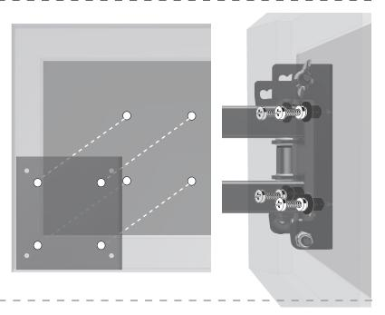
STEP 3 Install bracket with television to portable mounting plate: Attach as shown below.
