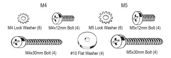
Hardware for securing bracket: Select the appropriate length based on the thickness of your mounting surface.
