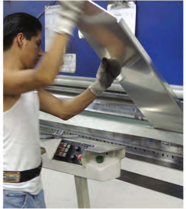
A MOR/ryde press brake operator bending a suspension part.
