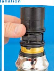
Pry each O-ring out to remove. Be careful not to damage the valve body.
