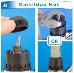
Using the grey assembly tool, pliers or a wrench, tighten the new 1255 cartridge nut until snug. Next turn approximately 90 degrees to fully secure the nut.
