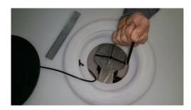
4. Grab pump by aluminum mounting plate and remove from tank.
