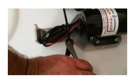
8. Remove handle mount screw from the top of the pump.
