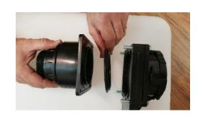
C. Using the original seal, assemble the 90-Degree plumbing to the discharge valve. You have the option to orienting the discharge in any direction you choose.
