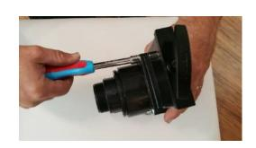
B. Separate the discharge valve as shown, keeping the seal in its original direction/orientation
