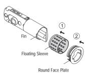
Locate floating sleeve and round face plate and proceed.
