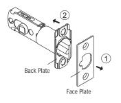
1. Use a flat screwdriver to separate the face plate.
