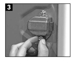
Place locking nuts on the bolts and hand-tighten.
