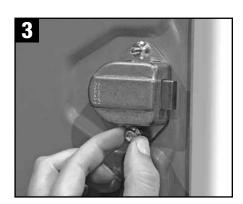
Place locking nuts on the bolts and hand-tighten.
