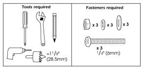
Mount may be installed on any angle horizontal surface. However, in order to use it as a rotating mount, it must be installed in a completely level position. Shims, not provided, may be used during installation to level this mount. Some fasteners required for installation.
