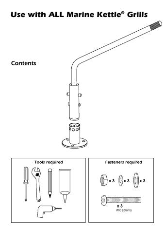
Mount may be installed on any angle horizontal surface. However, in order to use it as a rotating mount, it must be installed in a completely level position. Shims, not provided, may be used during installation to level this mount.
