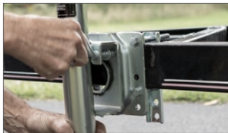
Heavy-duty pull-pin locks jack securely in place
