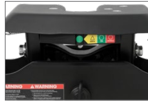
Three-position coupling indicator clearly shows coupling status
