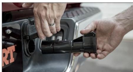
Insert Echo® between the vehicle and trailer
