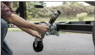
Swivel bracket allows jack to fully swing up during travel
