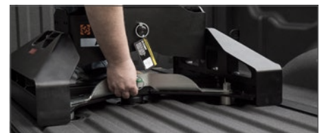
Step 3 - Secure levers with attached safety pins and you're ready to hitch up your trailer
