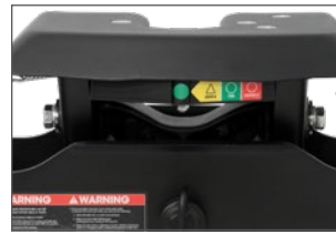
Three-position coupling indicator clearly shows coupling status
