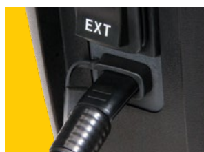
The 2-way plug inserts into the jack head underneath the control button.
