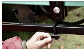
Adjustable brackets provide fixed support unlike chain models
