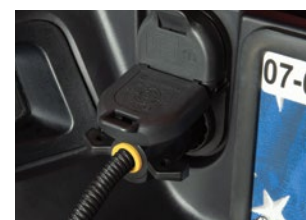
The 7-way plug inserts into the tow vehicle power receptacle on the back bumper.
