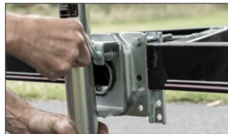
Heavy-duty pull-pin locks jack securely in place
