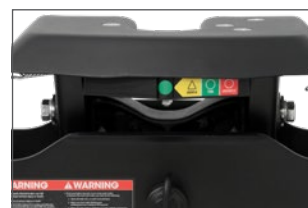
Three-position coupling indicator clearly shows coupling status
