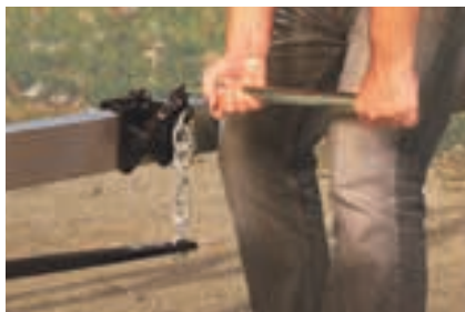
Standard weight distribution systems can require raising and lowering the tow vehicle with a jack over and over to get the right tension.
