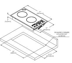
Overall Dimensions: 21" x 12" x 3" 533.4mm x 304.8mm x 76.2mm Cutout Dimensions: 20" x 10.75" with 1/4" radius 508mm x 273.05mm with 6.4mm radius
