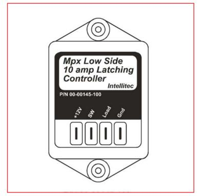
The MONOPLEXTM Water Pump Controller is designed to operate as a "low side", remote switch in 12 volt DC systems. As it's name implies, it was designed to control the domestic water pump. It's use, however, is not limited to that. It can also be used to control a variety of other loads such as lighting, other pumps, fans, etc., when it is convenient to switch the ground side.
