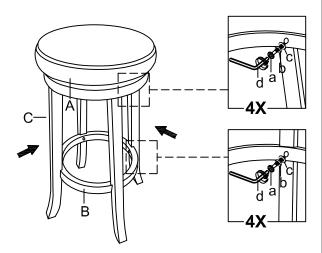
Attach part (A) with part (C). Tighten part (A) with part (C) first, then tighten part (B) with Part (C) completely.
