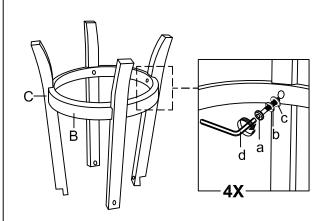
Attach part (B) with part (C). Insert each individual set of hardware as per picture shown. Do not tighten any hardware completely.
