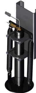
AP45660 Rear Jack Kit Two Straight-Acting (Power-Extend/Spring-Retract) Jacks with a lifting capacity of 9,000 lbs. per jack and a 15" stroke
