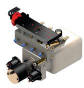
AP47564 Power Unit Kit 725 Series, 12 Volt DC Motor and Pump 125 amp - 3,000 psi relief with prewired control module and jack valving
