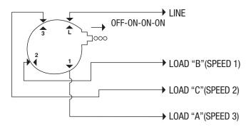
**NOTE:** This is a push-in / stab-type style switch. In order to insert the wires into the switch, you must have 18 AWG solid wire. If you do not have solid wire, you most solder the 18 AWG stranded wire together. You must be careful not to push the flap down to hard while inserting the wire as to much force will ruin the switch.
