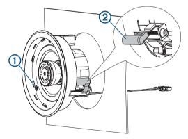
6 With the speaker mounted, place the grille onto the speaker, and push to secure it.
