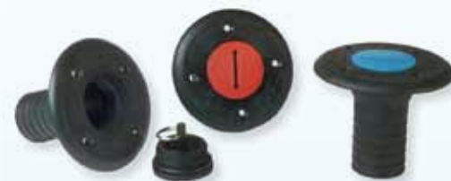
Deck Flange is 4"(101.6mm) dia. Cutout: 2-1/8"(53.97mm). Hose Barb Length: 3"(76.2mm).
