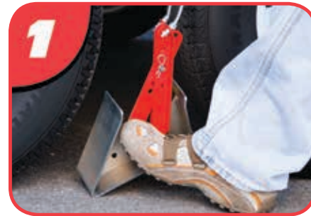
Use your foot to spread the chocks between the tires.
