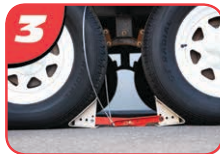
Lean the cable handle on the tire and you're done.
