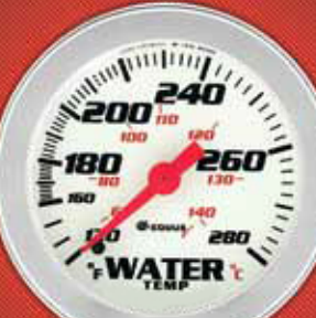
8442 2-5/8" Mechanical Water Temperature Gauge // 130° to 280° F / 60° to 140° C // 270° Full sweep for increased visibility // Comes with 72" (6') tube
