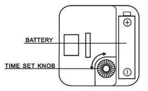
**Battery**: Insert one new 'AA'Alkaline battery according to the polarity marks in the battery compartment.
