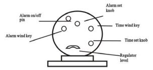
**To Set Time:** Turn the time set knob to the correct time. Wind the time key fully in the direction the arrow indicates.
